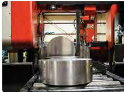
We offer bar sawing and can cut bar stock up to 32" diameter round.
